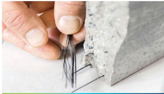
◀ Carbon prestressed concrete, reinforced with prestressed carbon fibers
